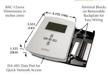
NOTE: Two-piece design allows field rough-in and termination of field wiring to the backplate without needing the FlexStat at the site—permitting FlexStats to be bulk-configured off-site and plugged into the wired backplates at a later time if desired.
