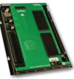
the controller is a BACnet router, a web server, and expandable I/O.
